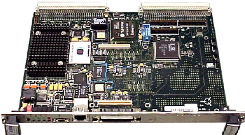
**The Power7E** (P7E) is a 6U VME 64 Single Board Computer. It is available with up to 256MB of ECC SDRAM. An additional 256MB may be installed via a mezzanine memory card for up to 512MB total system memory. In addition, the P7E contains 4MB of Intel Strataflash, 32kB of NVRAM, and 512kB of socketed flash memory. The P7E operates in either a system or a non-system slot.
